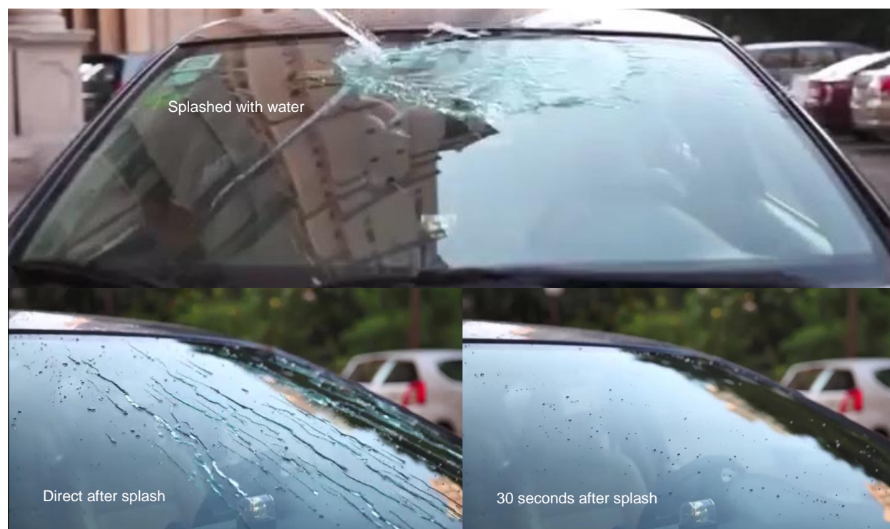
Figure 13. Effect on car windscreen of high contact angle coating (E. CV), full water repellence. Tilt angle of windscreen 25°.
