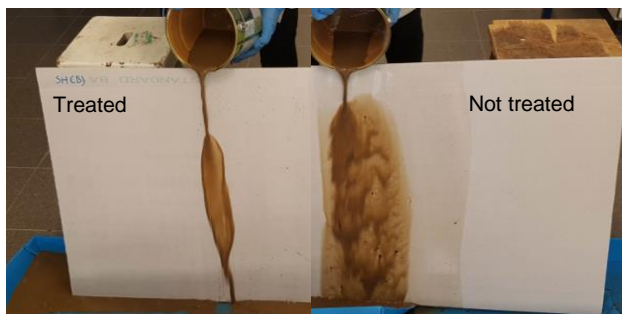
Figure 14. Superhydrophobic gypsum, left side treated with E. SH, right side not treated
