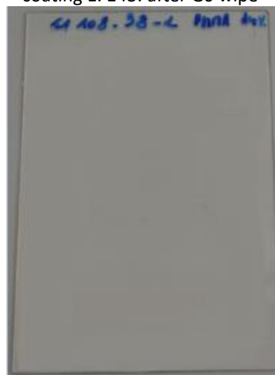
PMMA coated with anti-graffiti coating E. 143: after G0 wipe
