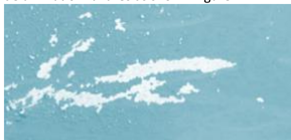
Figure 2. Example delamination fluorine based coating on metal
