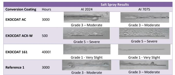
Table 5. Salt spray test of total system: conversion coating/epoxy/PU coating
