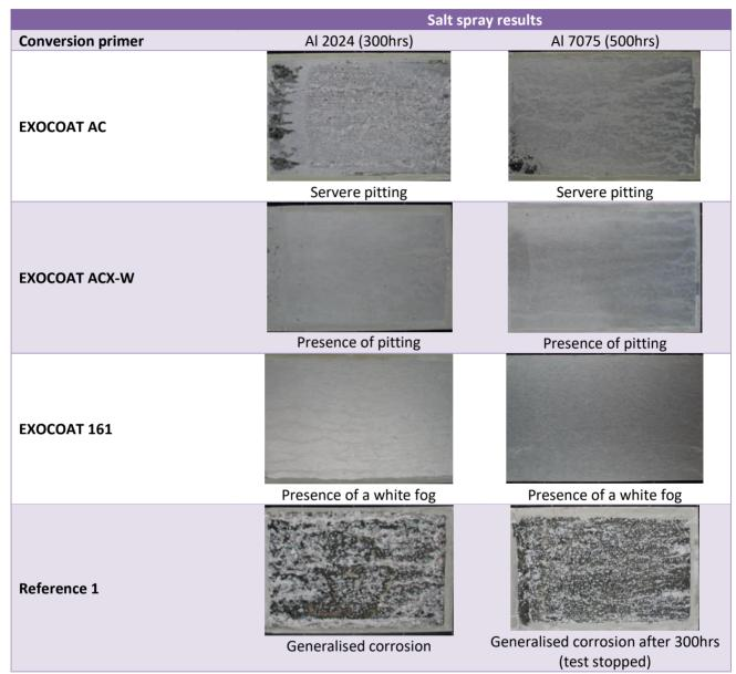
Table 4. Neutral salt spray test of monolayer (direct to metal)
