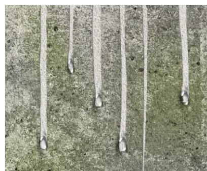
<Figure 1. A render exposed to a soiling test. A=untreated, B=EXOCOAT SH, C=an alternative treatment.
