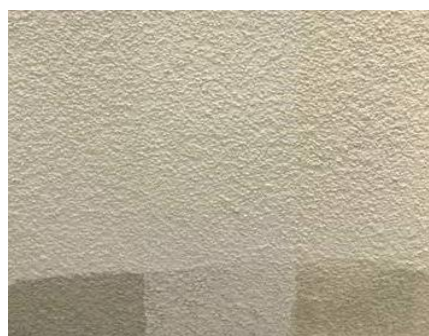
<Figure 1. A render exposed to a soiling test. A=untreated, B=EXOCOAT SH, C=an alternative treatment.
